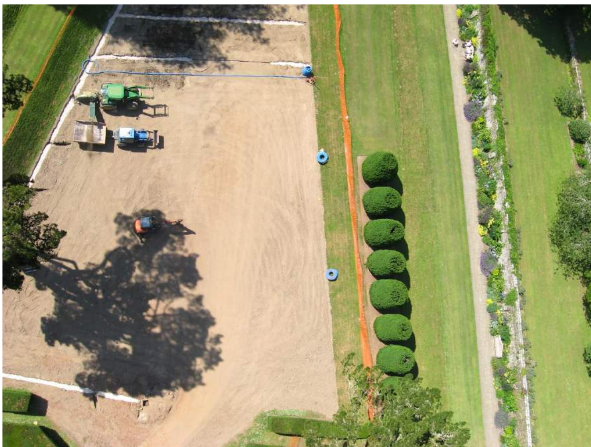
Figure 3 Updating herringbone drainage system through the base of the Tiltyard, 23.06.2009
